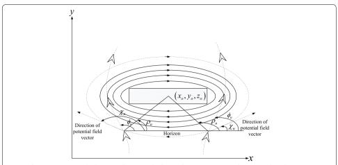
**Fig. 4** The trajectories in clockwise and counterclockwise direction respectively on x–y plane base on potential field with rotational vectors
