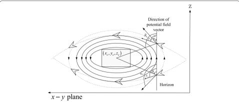
**Fig. 5** Rotational field with rotational vectors in upward direction and the downward in clockwise and counterclockwise direction respectively on y–z plane
