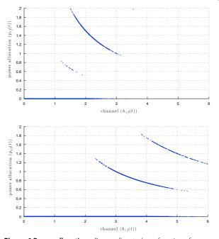
**Figure 6 Power allocations.** Power allocated as a function of channel realization is shown for channels with average power  $\mathbb{E} h_{if}(t)=1$  (top) and  $\mathbb{E} h_{if}(t)=2$  (bottom). The resulting power allocation is opportunistic in that power is allocated only when channel realizations are above average.
