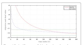
**Figure 4 Optimal frequency division broadcast channel.** Objective value  $\sum_{i=1}^{J} U_i(\bar{c}_i(t))$  and dual function's value  $g(t) := g(\boldsymbol{\lambda}(t), \boldsymbol{\mu}(t))$  for the algorithm in (93)–(97) are shown along with lines marking optimal utility and 90% of optimal yield. Utility yield becomes optimal as time grows.
