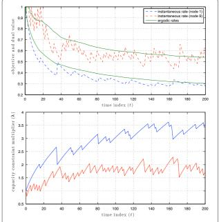
**Figure 3 Primal and dual iterates in dual stochastic gradient descent.** Evolution of dual variables  $\lambda_i(t)$  and rates  $r_i(t)$  for representative nodes with average channels  $\mathbb{E}h_1(t)=1$  and  $\mathbb{E}h_9(t)=3$  for the algorithm in (93)–(97) are shown. Multipliers  $\lambda_i(t)$  and capacities  $c_i(t)$  do not converge, but ergodic rates  $\bar{c}_i(t)$  do.
