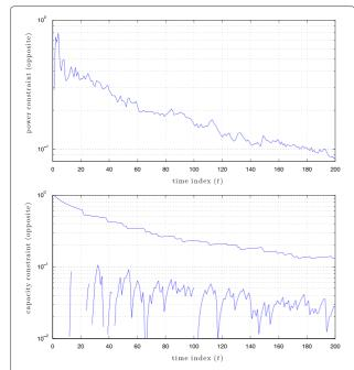
**Figure 5 Power and capacity constraints.** Feasibility as time grows is corroborated for the power constraint in (27) (top) and rate constraints in (26) (bottom). For the rate constraint we show the maximum and minimum value of constraint violation.
