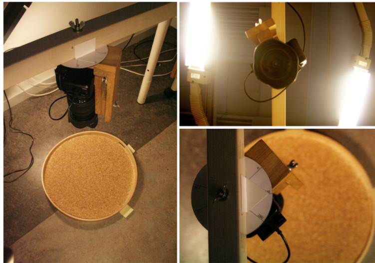
Fig. 2 The texture dataset image acquisition setup. From left to right : overview, view from the camera towards the texture surface beneath, view from the texture surface towards the camera and lights
