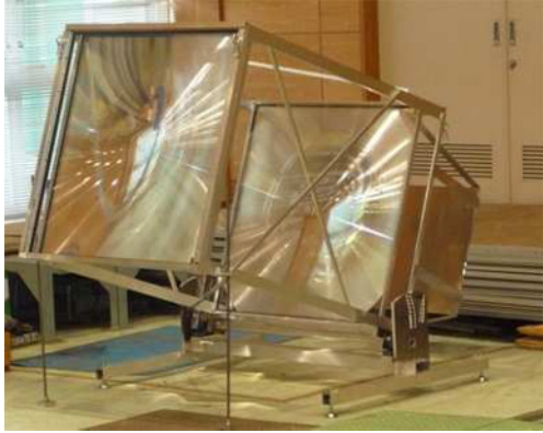
Figure 9. Photograph of the lenses system which will be used for TA-EUSO.
