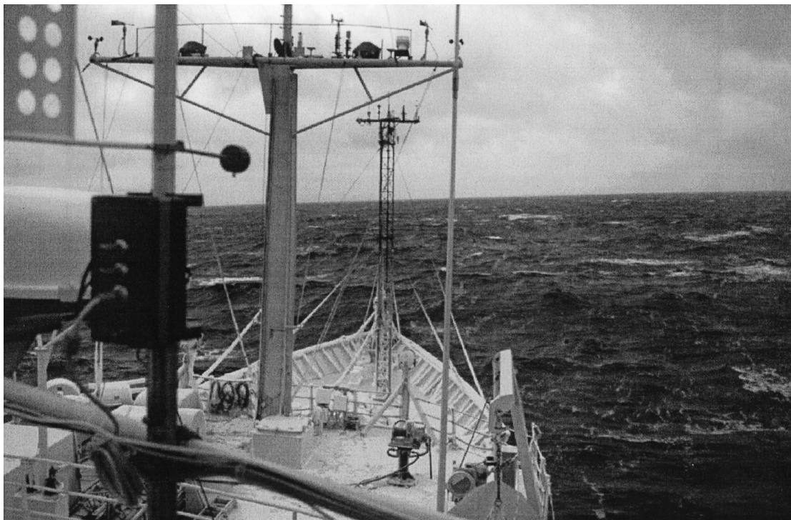
FIG. 2. Photo of the foremast of R/V Knorr taken from the observation deck. Instruments for turbulence measurements are mounted on the t-bar of the bowmast at a height of approximately 18.5 m above sea level. The foremast, which is approximately 11 m behind the bow mast, carries temperature and wind speed sensors of the ship's IMET.
