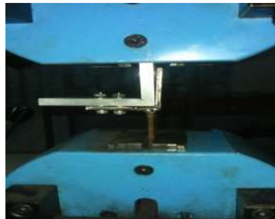
Fig 19. Tensile testing process with jig fixture
