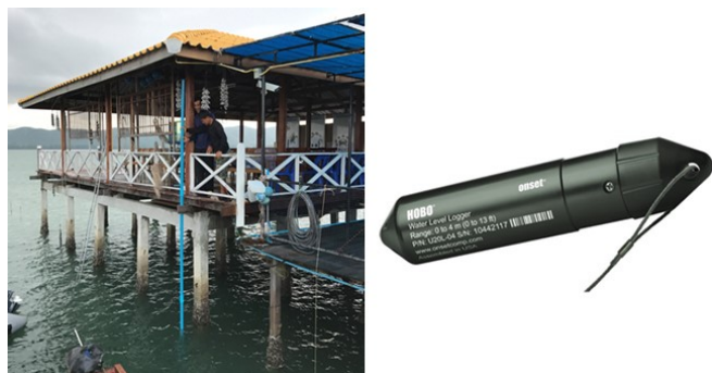
Fig. 3. HOBO water level logger and its deployment methodology for the water level variation survey between 24th April and 13th May 2017
