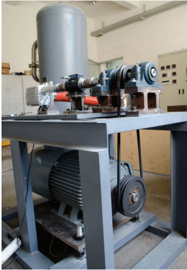
FIGURE 9: Twin-screw supercharger noise signal acquisition laboratory bench.
