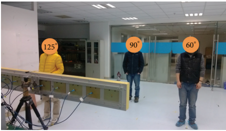
FIGURE 11: Experimental scenario for respiration detection of three human targets.
