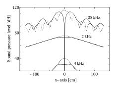
**FIGURE 1.** Propagation curves on the beam axis (left) and beam patterns at 4 m (right) for an ultrasound source consisting of two strip emitters with 10 cm width. The primary frequencies are 26 kHz and 28 kHz. The sound pressures on the source are 125 dB for both the primary waves. Solid and dotted curves denote the numerically obtained data for the out-of-phase and in-phase excitations, respectively.
