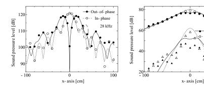
**FIGURE 2.** Beam patterns at 4 m from the source for the primary waves of 28 kHz (left). The patterns for the difference wave of 2 kHz and its second harmonic of 4 kHz are also shown (right). Symbols are all measured data, and solid and dotted lines are the theoretical predictions.
