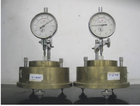
FIGURE 2: WZ-2 dilatometer used in swelling test.
