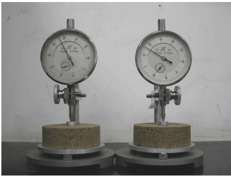
FIGURE 3: SS-1 contractometer used in shrinkage test.
