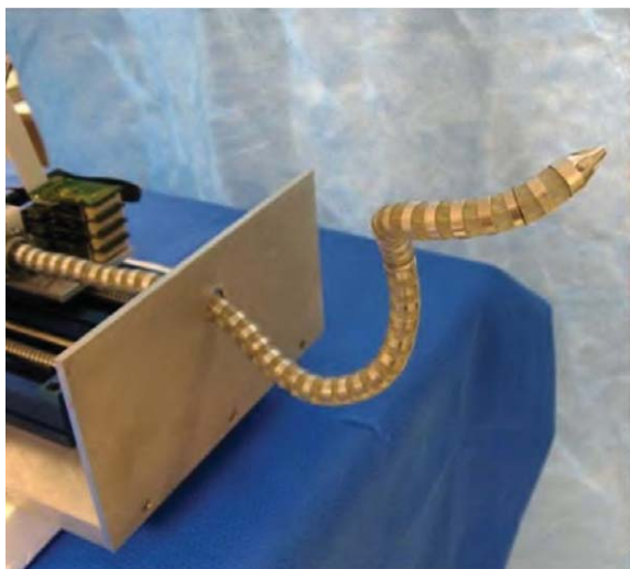
Fig. 3. 3D trajectory followed by the CardioARM™ developed by Cardiorobotics, Inc. [36] (© [2008] IEEE).
