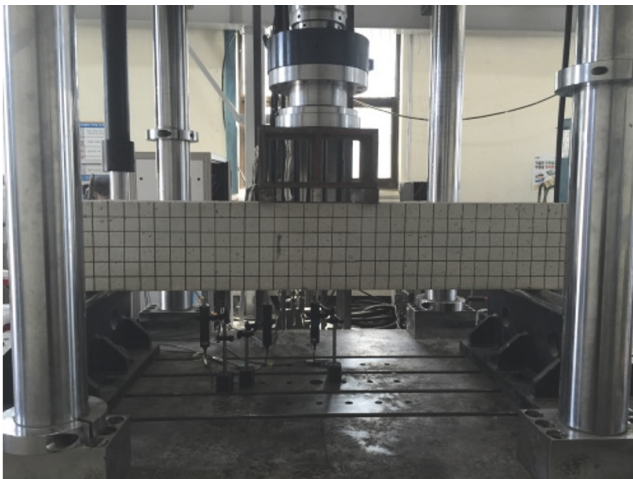
FIGURE 3: Setup for flexural test of AAS concrete beam specimen.
