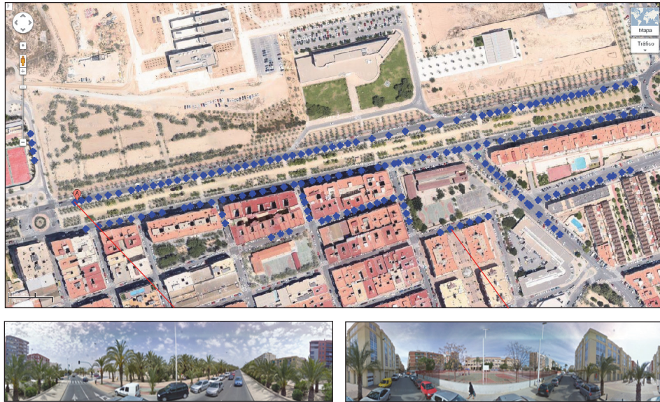
FIGURE 1: Bird eye's view of the region chosen as map 1 prior to the localization experiment. The blue dots represent the coordinates where the images of the Set 1 were captured. Two examples of Google Street View images after a preprocessing step are also shown.
