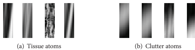
FIGURE 7: Example of (a) tissue atoms and (b) clutter atoms in the obtained subdictionaries from applying MCA with a cut-off value of \beta = 0.75 . The dictionary is learned using the simulated sequence echo data. The magnitude of the atoms is presented. The atoms are shown after being transformed from vectors into 2D patches and being envelope-detected. The horizontal direction refers to the temporal dimension and the vertical direction to the axial dimension.
