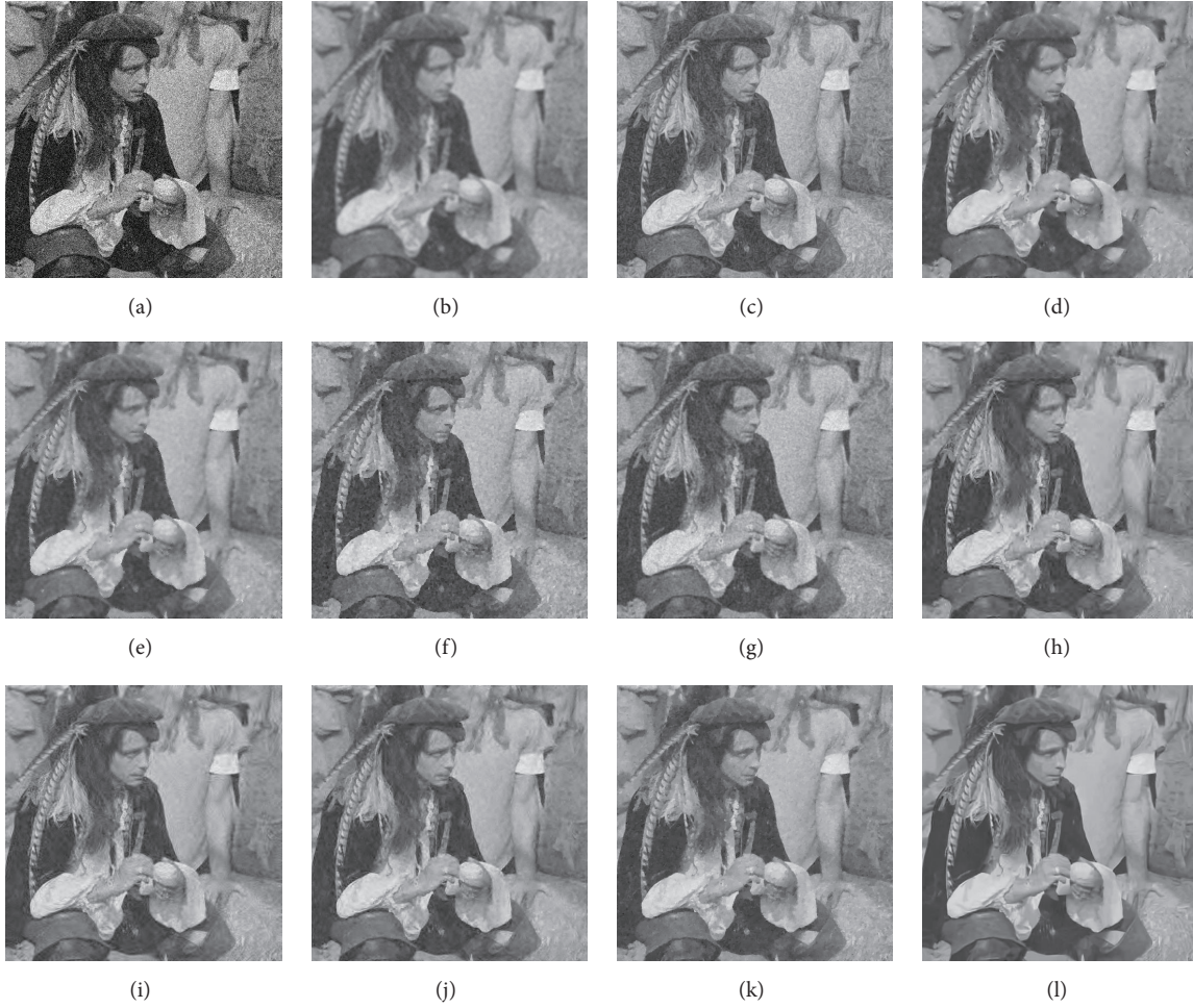
FIGURE 5: Comparison of the eleven denoising methods: (a) Noisy “Pirate” image with \sigma = 30 ; (b) bilateral filter; (c) structure adaptive kernel; (d) the proposed method; (e) Wiener filter; (f) Kuwahara filter; (g) NCD method; (h) BiShrink; (i) NeighShrinkSURE; (j) OWT-SURELET; (k) FP 2 O-ITV; (l) BM3D.
