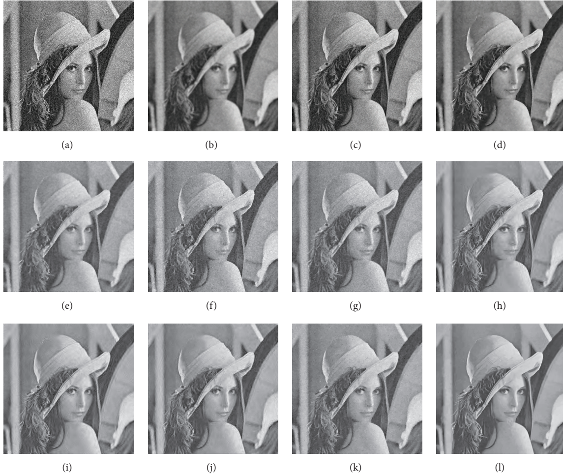
FIGURE 4: Comparison of the eleven denoising methods: (a) Noisy “Lena” image with \sigma = 30 ; (b) bilateral filter; (c) structure adaptive kernel; (d) the proposed method; (e) Wiener filter; (f) Kuwahara filter; (g) NCD method; (h) BiShrink; (i) NeighShrinkSURE; (j) OWT-SURELET; (k) FP 2 O-ITV; (l) BM3D.
