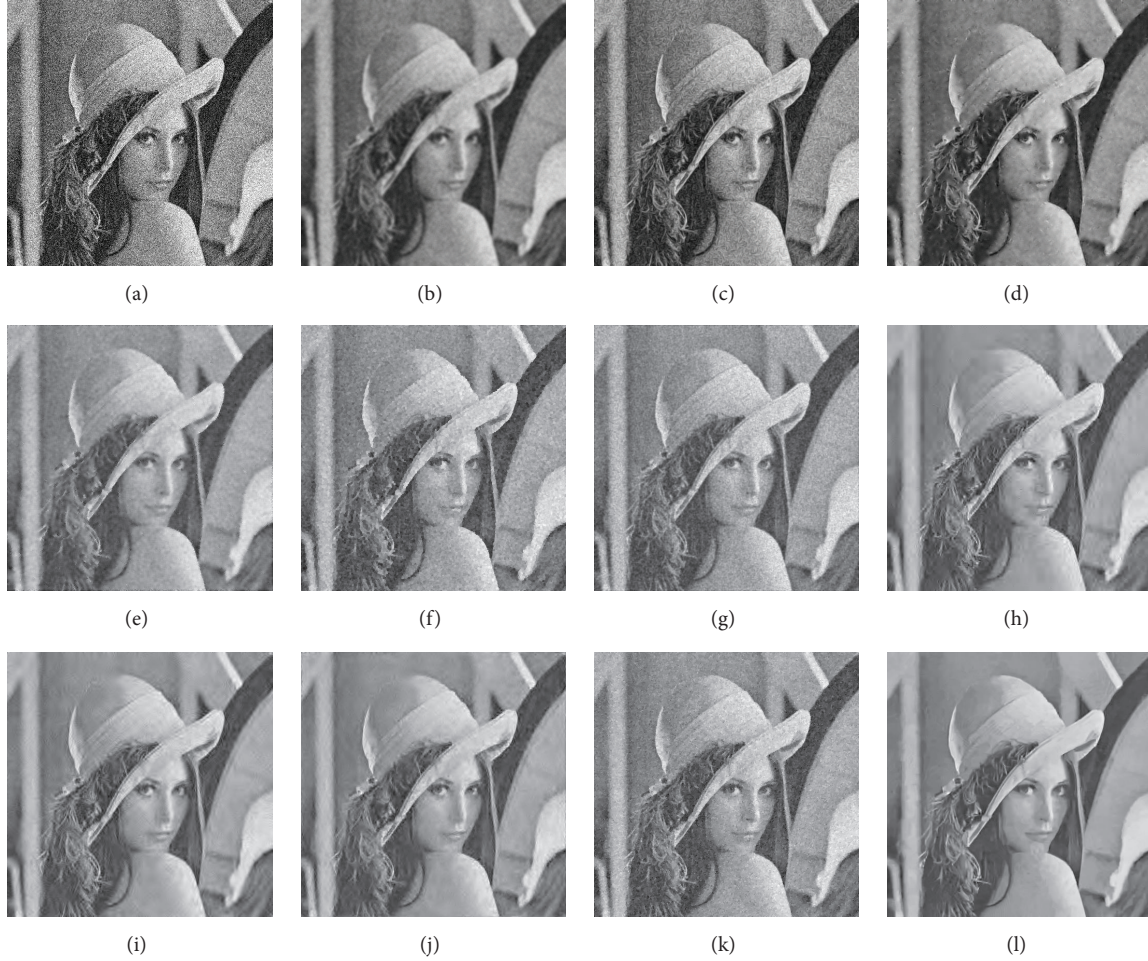
FIGURE 6: Comparison of the eleven denoising methods: (a) Noisy “Lena” image with \sigma = 40 ; (b) bilateral filter; (c) structure adaptive kernel; (d) the proposed method; (e) Wiener filter; (f) Kuwahara filter; (g) NCD method; (h) BiShrink; (i) NeighShrinkSURE; (j) OWT-SURELET; (k) FP 2 O-ITV; (l) BM3D.
