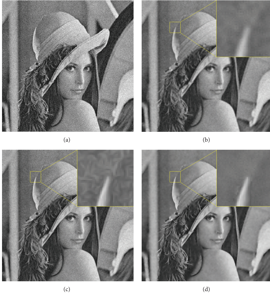
FIGURE 2: Comparison of the three denoising methods: (a) noise image with \sigma = 20 , (b) bilateral filter, (c) structure adaptive filter, and (d) the proposed method.
