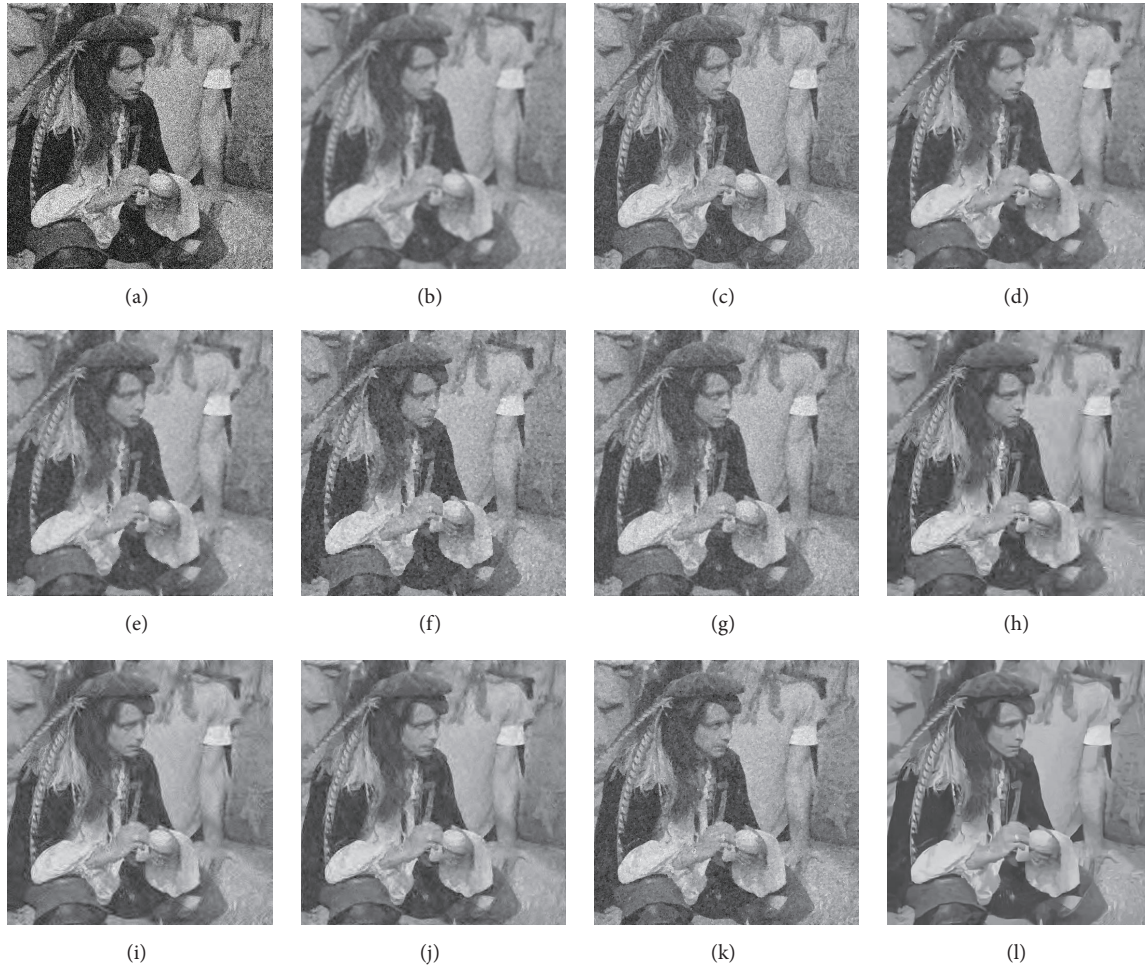
FIGURE 7: Comparison of the eleven denoising methods: (a) Noisy “Pirate” image with \sigma = 40 ; (b) bilateral filter; (c) structure adaptive kernel; (d) the proposed method; (e) Wiener filter; (f) Kuwahara filter; (g) NCD method; (h) BiShrink; (i) NeighShrinkSURE; (j) OWT-SURELET; (k) FP 2 O-ITV; (l) BM3D.
