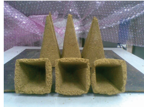
FIGURE 8: Fabricated hollow pyramidal parts of the absorbers, without a square base part, height (11 cm), and average wall thickness of 10 mm.
