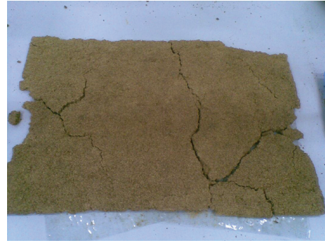
FIGURE 10: Propagation of crack due to the effect of high contents (greater than 70%) of the rice-husks on the structural stability of the rice husk-UPR composite.
