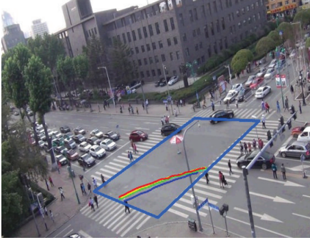
FIGURE 2: Extraction of left-turning vehicles' trajectories schematic diagram.
