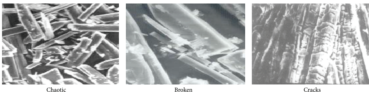
FIGURE 6: Plank and pillar-like gypsum crystal after SAV-1/SAV-2 treatment.
