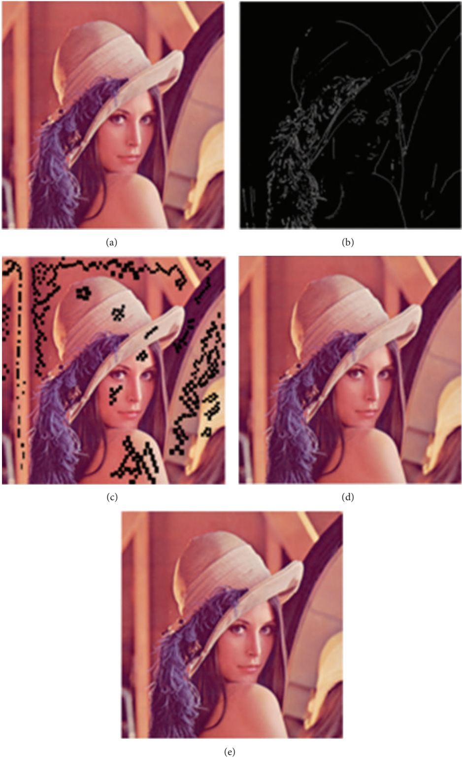
FIGURE 6: Comparison with JPEG 2000 with QP = 75. (a) Input image. (b) Edges. (c) Image with 25% of portions removed. (d) Reconstructed image after inpainting and texture synthesis. (e) Reconstructed image by JPEG 2000.
