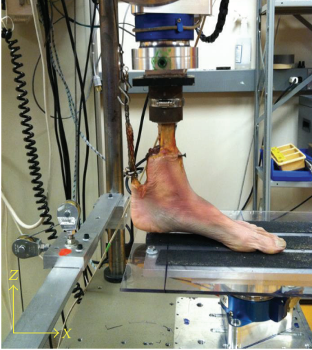
FIGURE 3: Specimen mounted in the RTP. This image shows clearance between the heel and X-Y table as the AT load is applied, allowing unconstrained arch formation.
