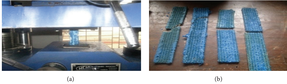
FIGURE 1: (a) Tensile testing; (b) tensile fracture samples of woven jute FRP.
