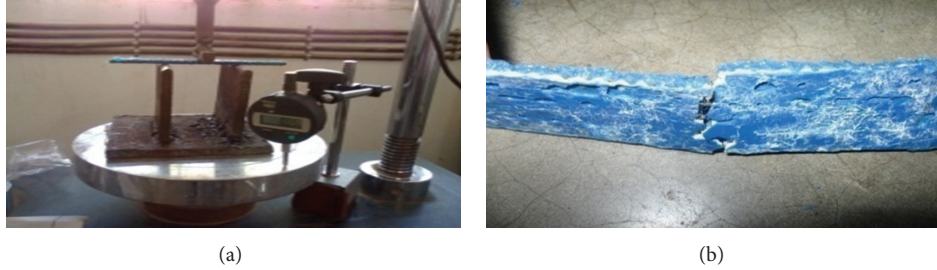
FIGURE 2: (a) Flexural testing; (b) flexural fracture of woven jute FRP.
