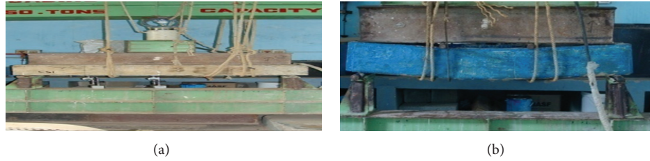
FIGURE 6: (a) Two pint loading system on a 50 ton loading frame; (b) loading on fully wrapped beam with woven jute FRP.
