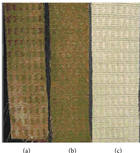
FIGURE 9: Antidust performance of polyester fabric. (a) Titanium dioxide coated fabric after flow of dust, (b) uncoated fabric after flow of dust, and (c) initial fabric before flow of dust [45].
