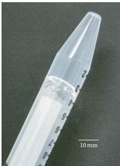
FIGURE 2: An appearance of the obtained imogolite hydrogel.
