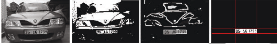
FIGURE 7: License plate segmentation steps.
