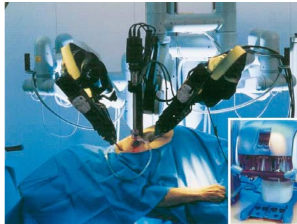
FIGURE 1. The da Vinci surgical system (Intuitive Surgical, Sunnyvale, CA) consists of a central arm that controls the laparoscope and camera as well as two side arms that are used to control a variety of grasping and cutting instruments. The surgeon can activate either the two side arms to direct the instruments or the central arm to adjust the surgical view. (Figure reprinted from Surgical Endoscopy 18(12) , 1694–1711, 2004. With kind permission of Springer Science and Business Media.)
