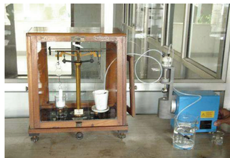
FIGURE 1: Modified two pan balance used for in vitro mucoadhesion studies.
