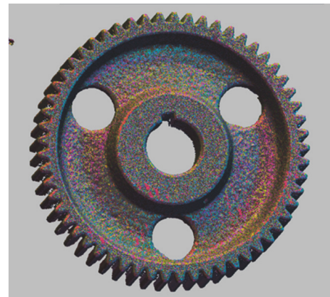
FIGURE 5: Edited point cloud before combining and sampling.
