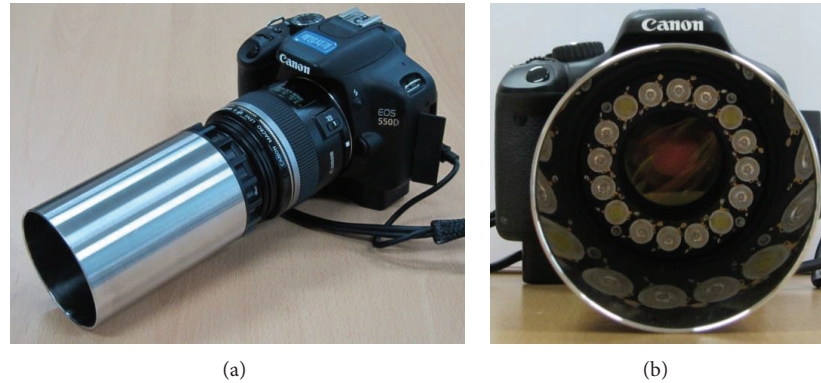
FIGURE 1: The QLF-D Biluminator used in this study. This device (a) is based on a full-sensor SLR camera (Canon 550D) equipped with an illumination tube with white and blue light-emitting diodes positioned in a ring around the lens opening (b).
