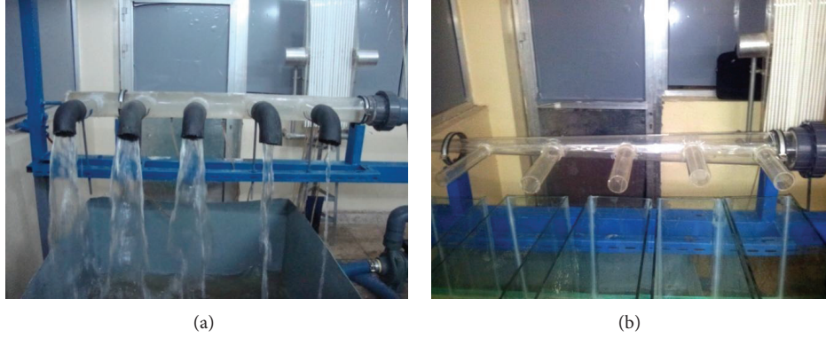
FIGURE 3: Experimental setup of two manifold configurations: (a) manifold with uniform longitudinal section and (b) manifold with tapered longitudinal section.
