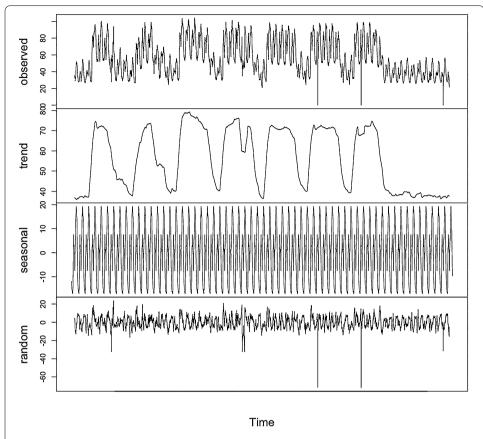
**Figure 3 Energy consumption time series decomposition for a residential area.** The *x*-axis shows the temporally sampled electric current flowing through the distribution lines recorded every 10 minutes. The *y*-axis reports the electric current passing through a given power line measured in Ampère at a given time. Monday is the first day of the week.
