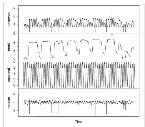
**Figure 5** Energy consumption time series decomposition for a city center/industrial. The *x*-axis shows the temporally sampled electric current flowing through the distribution lines recorded every 10 minutes. The *y*-axis reports the electric current passing through a given power line measured in Ampère at a given time. Monday is the first day of the week.
