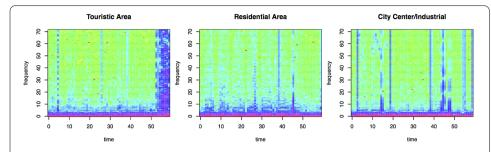
**Figure 2 Spectral characteristics of typical energy consumption response variables.** The units reported in the temporal *x*-axis are days (the temporal scaling was done starting from the 100 milliseconds initial resolution), while the vertical axis represents frequency. The amplitude of a particular frequency at a given time is given by the intensity and the color of each point in the plot.
