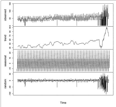
**Figure 4** Energy consumption time series decomposition for a touristic area. The *x*-axis shows the temporally sampled electric current flowing through the distribution lines recorded every 10 minutes. The *y*-axis reports the electric current passing through a given power line measured in Ampère at a given time. Monday is the first day of the week.
