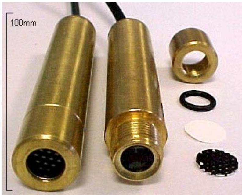
FIGURE 1. The sub-surface fuel sensor. The sensor on the right shows an exploded view of the sensor head assembly, exposing the NIR photoemitter/detector situated behind the glass face of the sensor body.
