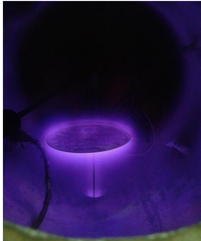
Fig. 1. Plasma Modification of nano-calcium silicate
