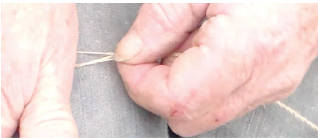
Figure 7. CTM(1): Twisting dried flax into twine.
