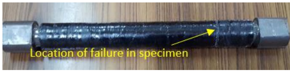
Figure 5: Failed specimen after torsional loading
