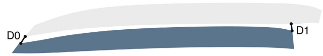
Fig. 7 A potential neighbour panel. The length of the new panel and the distances d1 and d2 are used to determine the new panel's suitability
