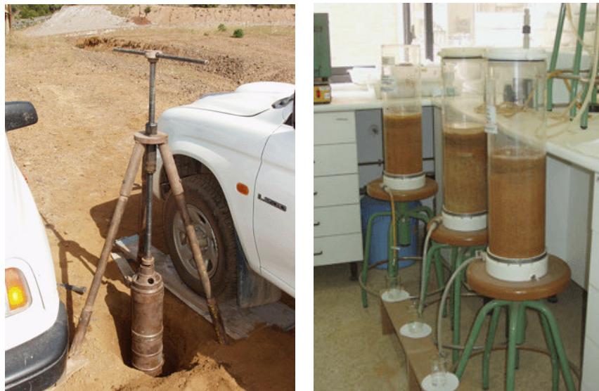
FIGURE 4. (Left) The system used for obtaining of undisturbed soil columns; (right) column leaching studies.
