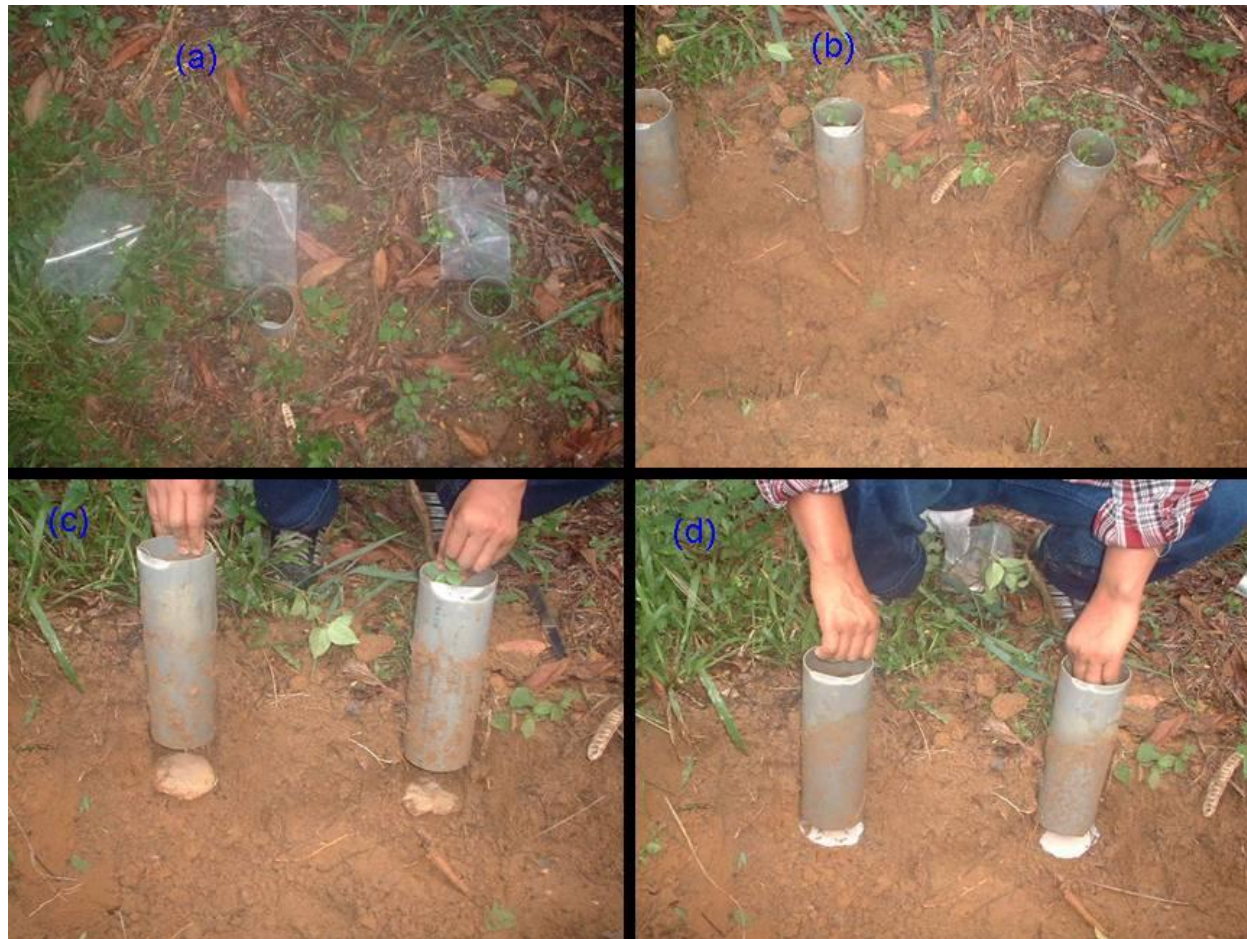
FIGURE 3. Sampling procedure showing (a) a view of the PVC tubes as inserted and sampling bags just before sampling, (b) tubes after excavation of surrounding soil showing position of resin bags, (c) old resin bags removed, and (d) replacement of old resin bags with fresh ones.
