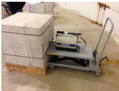
Fig. 2. Coaxial detector inside a standard cement blocks at Bessines.
