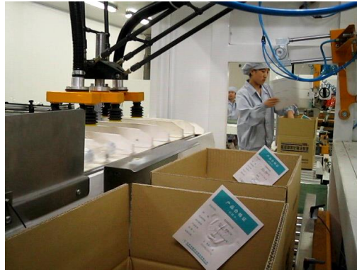
Fig. 6. Diamond robot used for packaging non-PVC transfusion bags
