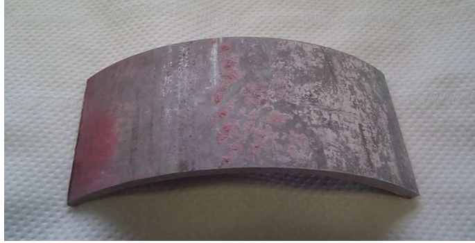
Figure 1.2: Pipework section that has undergone dye penetrant inspection; note the collections of penetrant around areas of rough surface which are liable to give a false defect indication.
