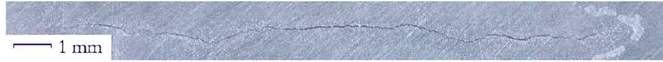
Figure 7.1: Image of artificially grown 3 mm deep defect in 10 mm thick stainless steel plate.
