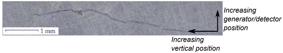
Figure 7.7: Image of the 1.4 mm deep defect used for raster scanning, showing the direction of the raster scan. The image has been rotated by 90^\circ to the left, relative to the image in figure 7.8 so as to fit on the page.
