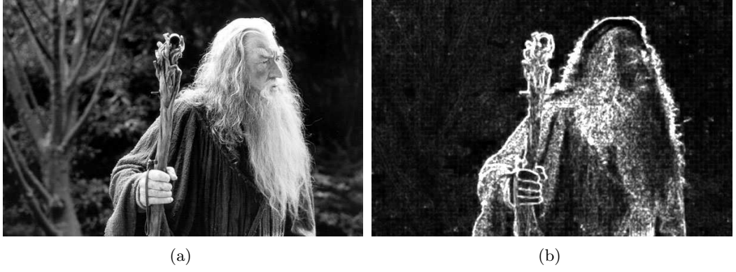
Figure 3.4: Low DoF image taken from video footage (a), and the corresponding focus intensity map generated using the SML method (b). The image has had its intensity enhanced by a factor of 3 for clarity.
