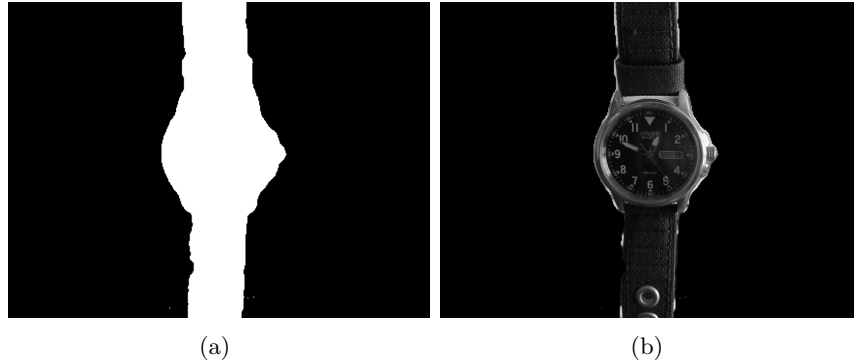
Figure 4.5: Object segmentation: (a) binary segmentation S(x, y) ; and (b) object segmentation I(x, y) .
