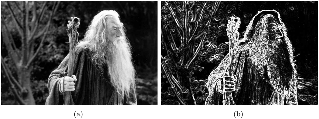
Figure 3.2: Low DoF image taken from video footage (a), and the corresponding focus intensity map generated using the Tenengrad method (b). The image has had its intensity enhanced by a factor of 3 for clarity.
