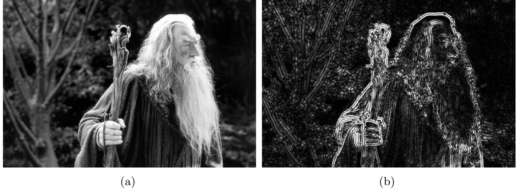
Figure 3.6: Low DoF image taken from video footage (a), and the corresponding focus intensity map generated using Daugman method (b). The image has had its intensity enhanced by a factor of 3 for clarity.
