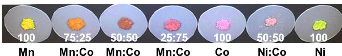
Figure 5.13: Colour change across the series of pure and mixed-metal materials.
