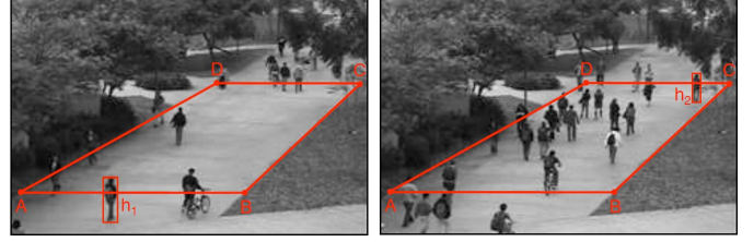
(a) Reference person at line AB. (b) Reference person at line CD. Fig. 3: Geometric correction for perspective distortion. Images from [7].
