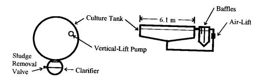
Figure 1. Top and side view of greenwater tank culture system.
