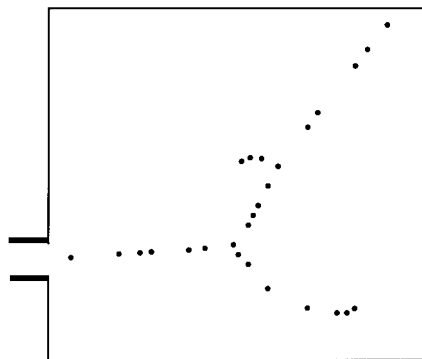
Figure 1. Particle trajectories in a bubble chamber. A particle that enters the chamber at the lower left creates microscopic bubbles as it encounters nuclei along its path. It splits to produce two continuing trajectories. The composite trajectory produced by all the ensuing particles in the presence of surrounding electric and magnetic fields identifies and characterizes the original particle and its descendants.
