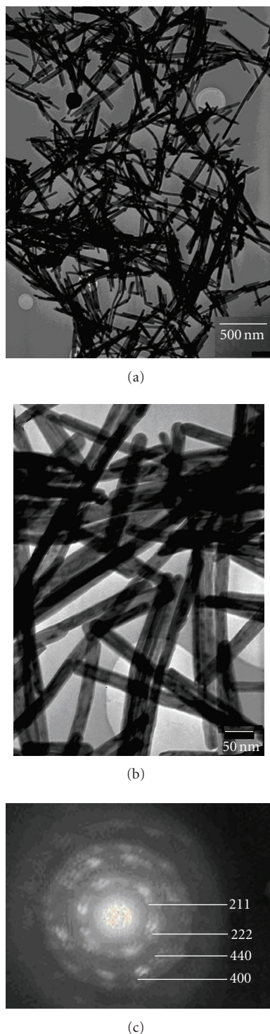
FIGURE 3: TEM images of the calcined samples ((a), low magnification (b), high magnification) with its SAED pattern (c).
