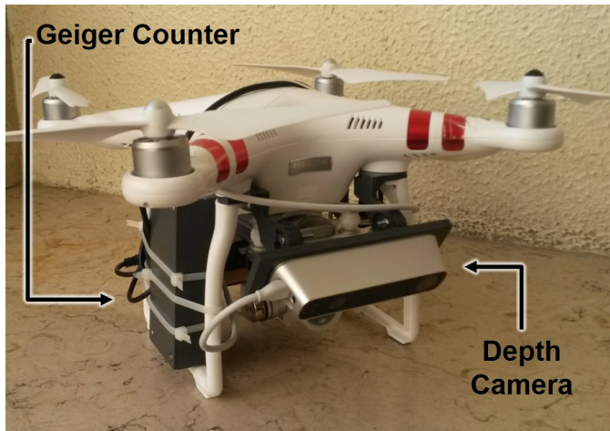
Fig. 11: Quadcopter equipped with a Sparkfun Geiger counter and a Structure depth camera.
