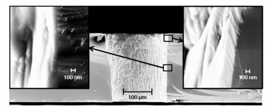
**Figure 3.** SEM cross-section through a via after deposition of 550 nm a-Si:H in a PECVD process. The a-Si:H thickness is 300 nm at via top (right) and below 100 nm at the via mid-position (left), respectively.
