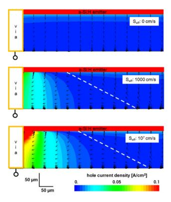
**Figure 7.** Hole current densities and vectors for different via surface recombination velocities for a  $100 \,\mu\text{m}$  via at the operation point of the cell. The vectors point in the direction of the conventional current flow.
