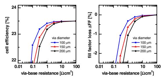
Figure 5. Simulated solar cell efficiencies and FF for different via-base resistances and different via diameters. Below 1  $\Omega$  cm<sup>2</sup>, the cell performance drastically decreases.
