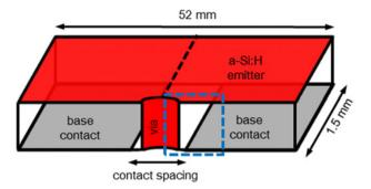
Figure 2. Cell geometry for 3D-simulation. The results are presented as 2D slices through the via (dashed area).
