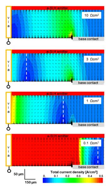
**Figure 4.** Current densities and vectors for different via-base contact resistances for a  $100 \,\mu\text{m}$  via at the operation point of the cell (simulated area as indicated in Fig. 2). The vectors point in the direction of the conventional current flow.
