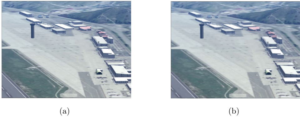
Figure 3.7: Example of Gaussian smoothing filter. Original image on the Left and smoothed image on the right
