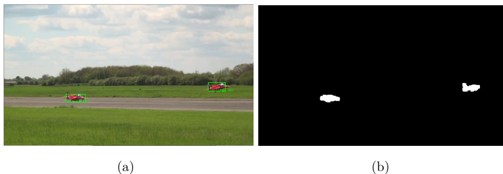
Figure 3.4: Example of colour segmentation. Figure (b) shows the binary image obtained by colour extraction and opening operator. Figure (a) shows the result on original image with a green rectangle on the object found.
